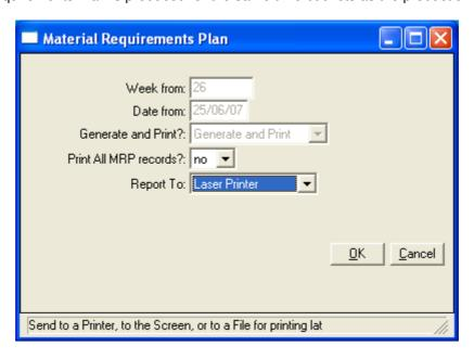
The MRP specifies the raw materials to be purchased and the parts to be manufactured to produce the finished products specified in the production schedule It gets the information it needs from the bill of materials set up for each manufactured product and part. The bill of materials specifies the purchased and manufactured parts required to manufacture a product or another manufactured part.
