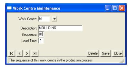
The work centre is assigned a sequence in the factory and a lead time for manufacture to assist with scheduling of production orders. In this case, Moulding is the first work centre, and whilst the process of moulding the polypropylene into a plastic dustpan or banister does not take very long, the manufactured parts have to dry and harden overnight, so the total time in the Moulding work centre is 1 day.
